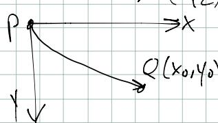
a) solve for  $\frac{dy}{dx}$ ,  $\Rightarrow 1 + \frac{dy}{dx}^2 = \frac{k^2}{y} \Leftrightarrow \frac{dy}{dx} = \pm \sqrt{\frac{k^2}{y} - 1}$  (take + root since + velocity)
