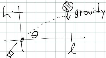
1) path of ball. We have that gravity  $\Rightarrow y(t) = h - \frac{gt^2}{2}$  (from rest)
